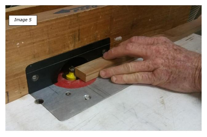
Wait until the box is assembled before cutting the handle to length. Place one end against the end and mark the other with a knife to give you and accurate length. Fix with a screw.
